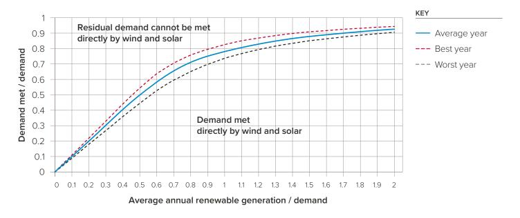
A) Fraction of demand that can be met directly by wind and solar in an average year.
