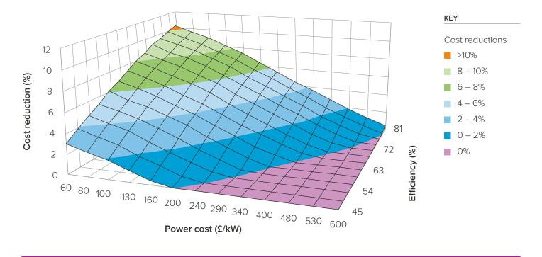
Example of storage parameters for hydrogen storage (base costs) together with ACAES, with compressor and expander costs of £340/kW and 66% round trip efficiency without contingency.
